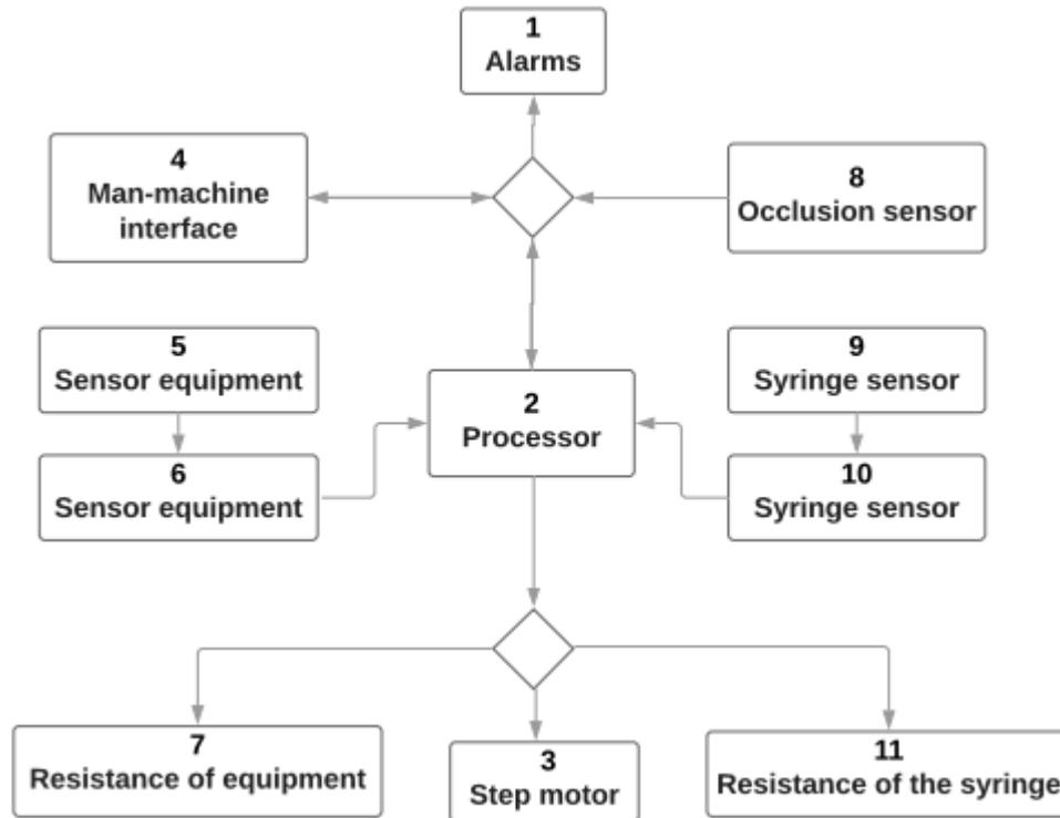
**Figure 3:** Electronic system flowchart.
