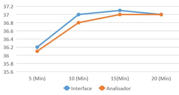
**Figure 2:** The graph shows the comparison of the prototype with the instrument calibration, the time it takes to reach 37 ° C.
