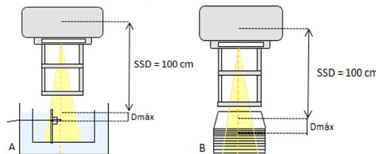
**Figure 3:  $F_{\text{output}}$  with radiochromic film and ionization chamber for square blocks**
