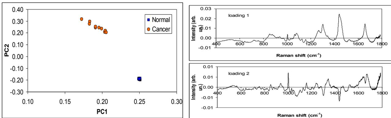
Figure 2 – Principal components scores (PC1 x PC2) and loading vectors (loading 1 and loading 2) extracted from the spectra of breast tissues.
