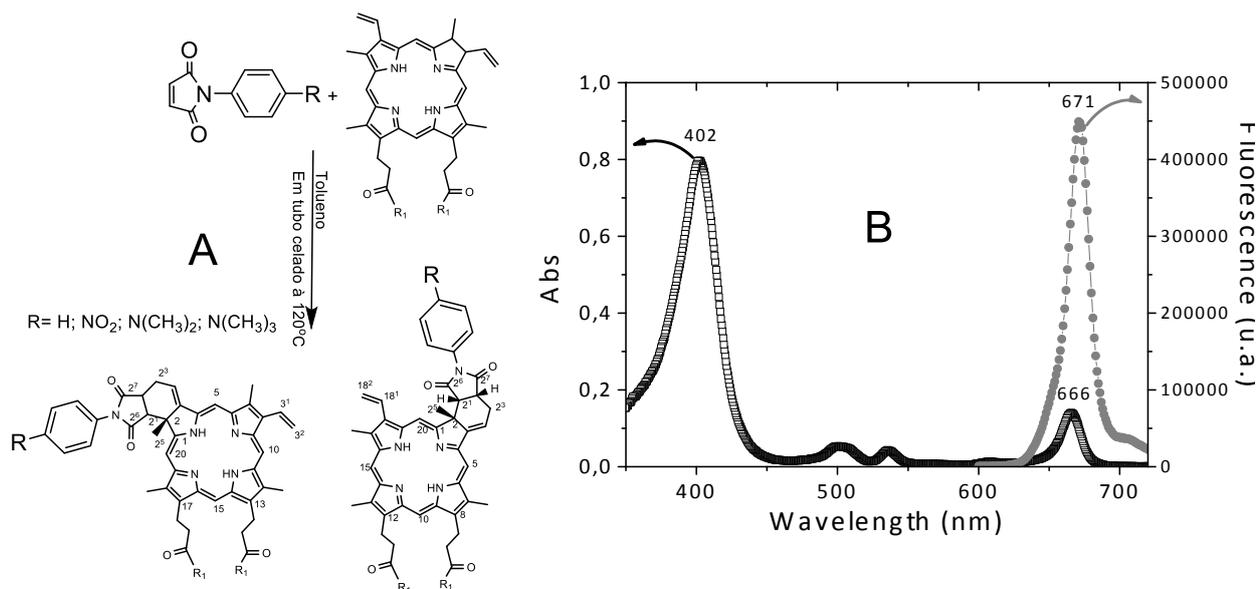
Figure 1: A) Synthetic route of new photosensitizer B) Absorption spectrum UV-Vis (left) of the new photosensitizer and fluorescence spectrum (right).
